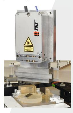
the resolution or stability of the measurement. The length resolution of the interferometer is 5 pm and this can be achieved even under normal laboratory conditions thanks to the differential principle of the measurement system.
